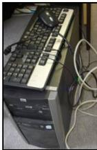
An HP Proliant ML310 Intel Pentium D tower style server with DAT 72 DDS tape drive, keyboard and mouse
