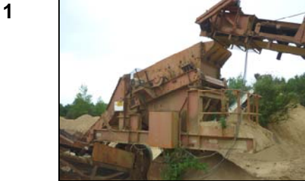
A Goodwin Barsby type 42 x 24 VLD Goliath mobile crushing machine, no. 29934 and type 8-0 x 4 0 MOB screening machine with three delivery conveyors
