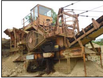
A Goodwin Barsby type 42 x 24 VLD Goliath mobile crushing machine, no. 29934 and type 8-0 x 4 0 MOB screening machine with three delivery conveyors
