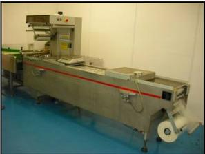
A Multivac M855 thermoformer with 'three-up' heated dye, sealing station with transverse and longitudinal cutting, vacuum suction and trim tank (REMOVAL METHOD STATEMENT REQUIRED) | £.....+BP+VAT |
